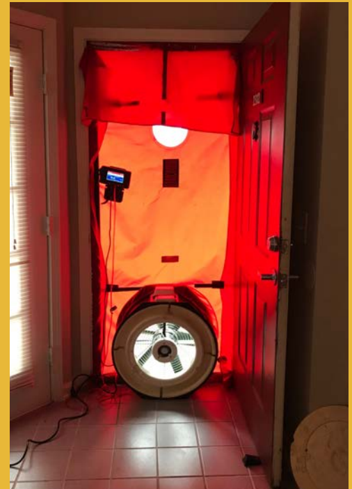
Blower door equipment, ready to measure the building envelope air leakage rate.
