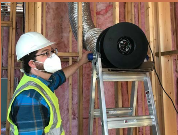
SK Collaborative verifier performs air leakage testing on a townhome development under construction using a duct blaster.
