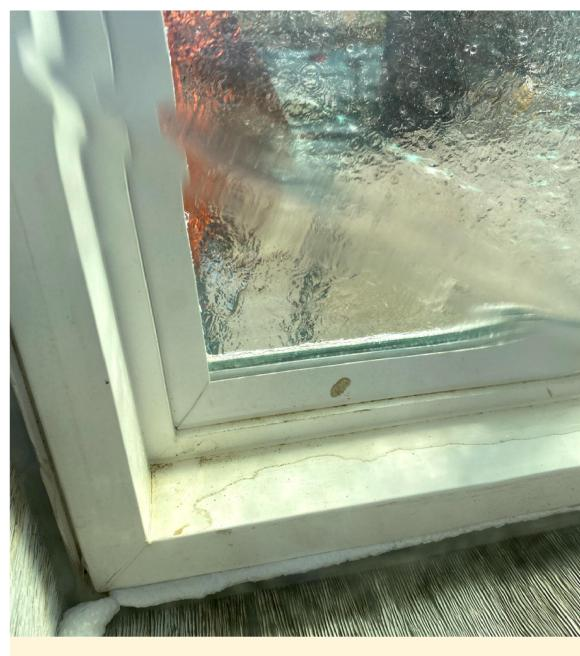
Now the test is up and running! Typically, we will run it about five times with breaks in between to check for leakage.
