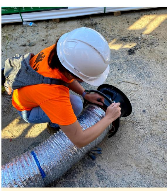
Here, the window is being sealed so that we can depressurize the chamber and isolate the window.
