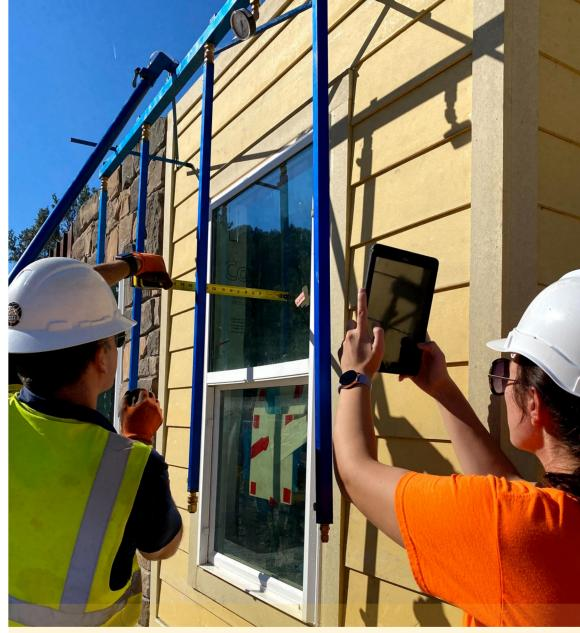
Insert the other end of the duct to the seal in the window. The green tube in the other opening is then connected to the pressure gauge.
